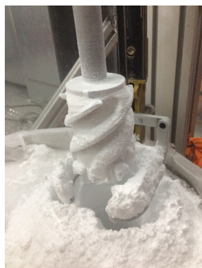
Figure 1. Drilling in cryogenic ice (unheated bit).
