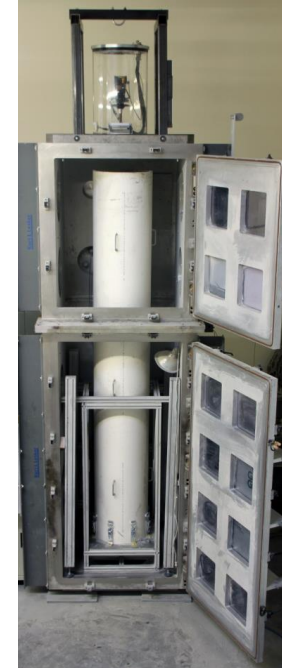
Pneumatic excavation in a vacuum chamber
