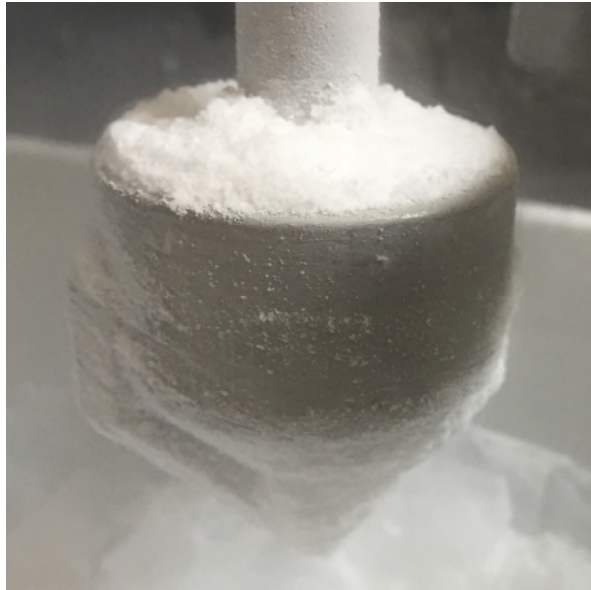
Figure 2: Close-up of the DRACO bit (DRill for the Acquisition of Complex Organics), 46mm in diameter, after drilling into frozen 30% ammonia solution (~ammonia dihydrate) ice at sub-100K temperatures. Satisfactory fine cuttings are generated.
