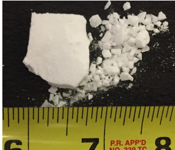
Figure 3: Close-up of the rotary-percussive cuttings from paraffin wax drilled at near 77K. Interestingly, a distinct 2-3mm particle size fraction dominates, although some finer particles exist
